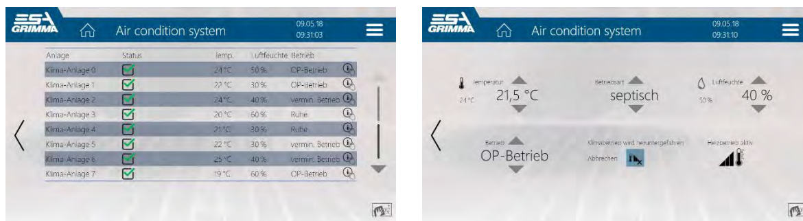
Fig. 14: left: trade overview “air condition system” right: trade view “air condition system” with all available control elements
