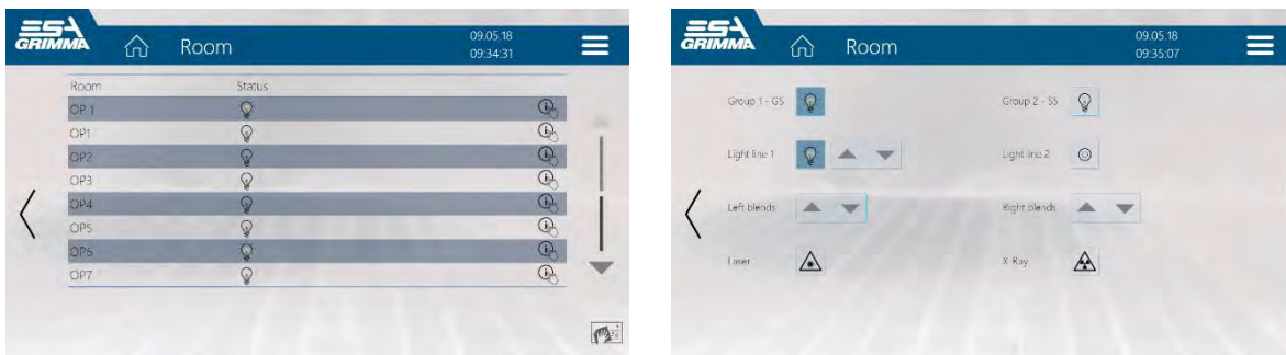
Fig. 12: left: trade overview “lighting” right: trade view “lighting” with all available control elements
