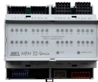
digital in- and output device MPM 32vario
