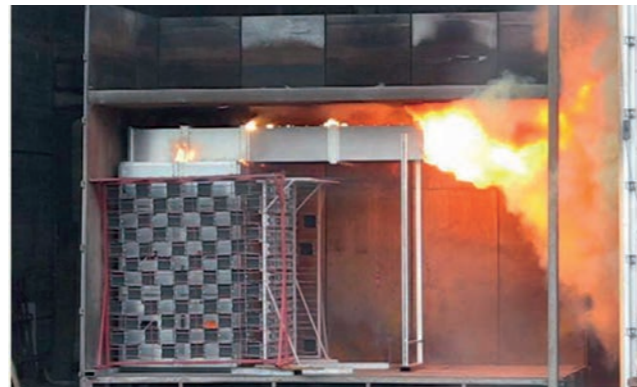
The arc fault testing for a medium voltage field with a pressure release channel
